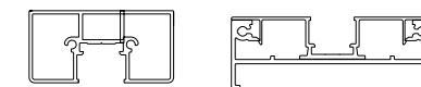
/ Minimal mullions (i.e., half), 40x80mm and 40x120mm, for framing upon an existing post.
