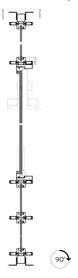
Fixed parts with hinged glass panel, corner and "T" shape construction
