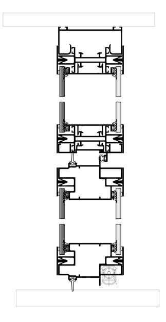
Vertical section of fixed walls and kicking plate (wiring)
