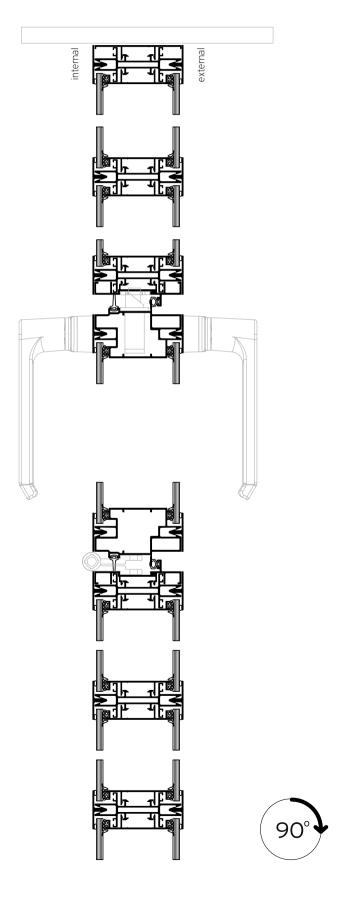
Fixed parts with hinged door panel and corner & "T" shape structures
